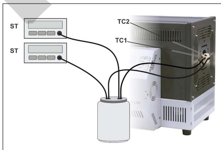
**Fig. 18 - Equipment Connections**
