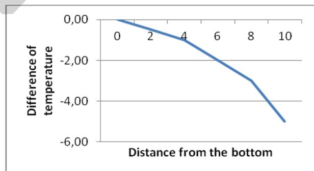
It is possible to observe in the example that as the sensor moves away from the bottom and approaches the top, there is a drop in temperature. In this case, increasing the value of the TOP setpoint it is possible to gradually reduce this temperature difference.
