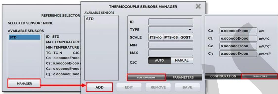
**Fig. 09** - Adding a new Reference Sensor
