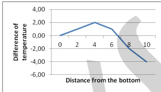
It is possible to observe in the example that as the sensor moves away from the bottom and approaches the top, there is a rise and then a drop in temperature. In this case, increasing the value of the TOP and BOTTOM set points it is possible to gradually reduce this temperature difference.
